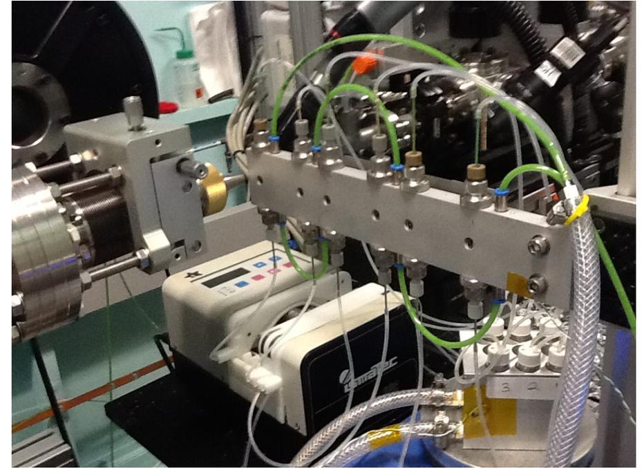
Multiple temperature controlled recirculation
