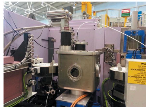
High field magnet with cryostat
